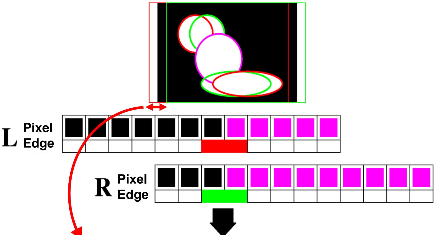
The offset at “two edges and minimum SAD” represents its depth
