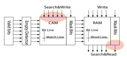
Reuse Buffer with Special Purpose CAM (One cycle for Search&Write and Search&Read)
