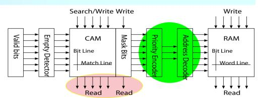
Reuse Buffer with General Purpose CAM (One cycle for Search, Write, and Read)
